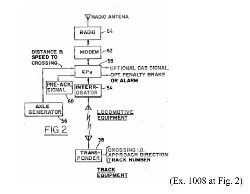
49. In particular, the message from the transponder contains data representing the identity of the upcoming crossing (i.e., crossing I.D.), the direction the
